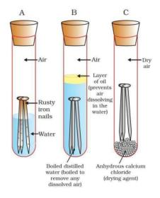
Put some anhydrous calcium chloride in test tube C and cork it. Anhydrous calcium chloride will absorb the moisture, if any, from the air. Leave these test tubes for a few days and then observe.
